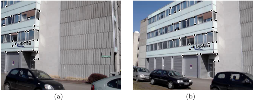
Fig. 7. The original common points in white together with their FACTMLE-EM reprojections in black. The two images are the first ones in the respective camera sets.
