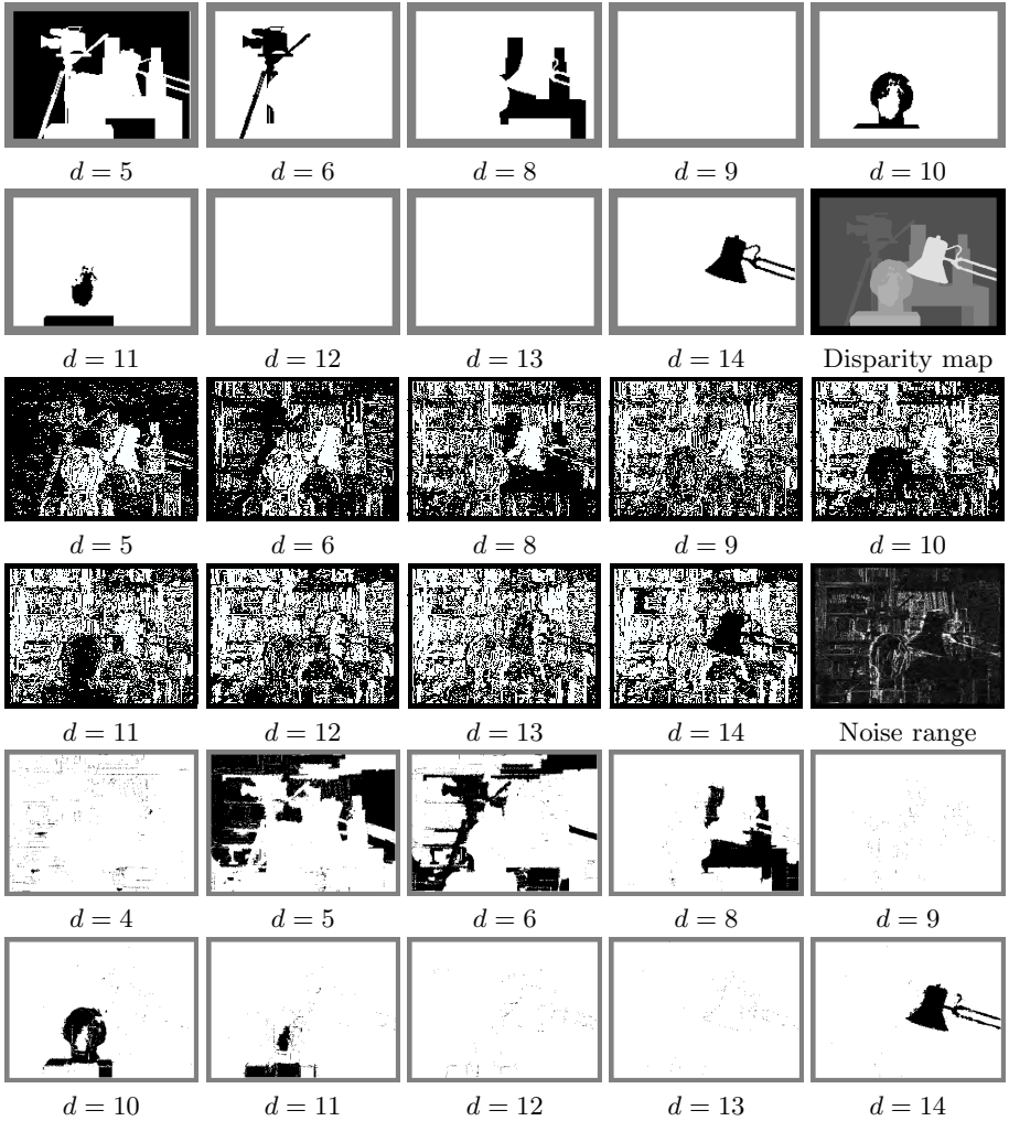
Fig. 3. Stereo pair “Tsukuba” – First two rows: Ideal disparity map for selected disparities d . Middle two rows: First nine panels: Candidate (x, y, p) volumes sliced at selected values of d . Large black regions clearly indicate good candidates for the final surfaces. Tenth panel: SDPS-estimated spatial noise variation – black-to-white coding of a noise range from [0,0] to [0,27] (white indicates the largest range). Last two rows: Selection of reconstructed surfaces.
